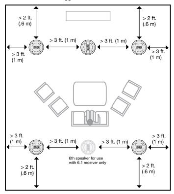
Refer to the Bose® *Virtually Invisible*® 791 series II and 591 in-ceiling speakers installation guide for installation instructions.
